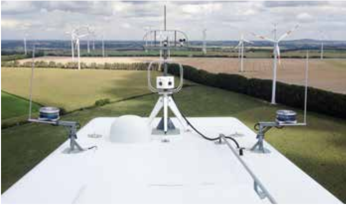
LiDAR Sensor Installed on Wind Turbine Nacelle
